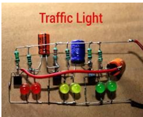
Traffic light circuit board with capacitors
