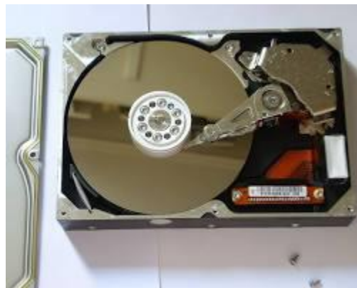
Hard drive showing magnetic platters
