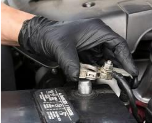
Cleaning battery terminals
