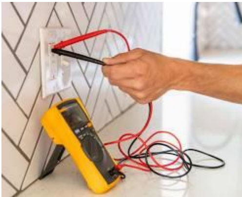
Person using a multi-meter to test a circuit
