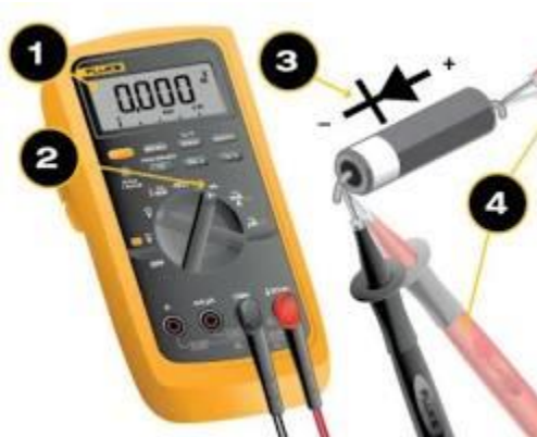
Multimeter testing a diode
